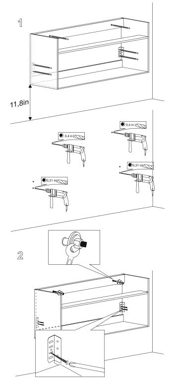
Step 2 Place the vanity frame on the finished wall and install at the locations drilled with the screws shown in Figure 2:
