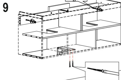
Only for 1973, 55in, install the bracket assembly. Version with set of 2 legs
